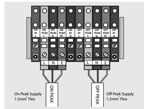
Clamp the cables in the grips provided and ensure all cables are routed to avoid hot surfaces.
